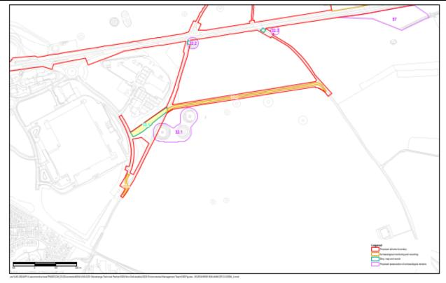
Site 33 comprises the proposed highway link between Allington Track and Equinox Drive and from the proposed AMES1 byway link between Equinox Drive and Amesbury Road. The Scheme proposals require the stopping-up of Amesbury Road and the closure of its connection with the A303 east of the Solstice Park junction.
