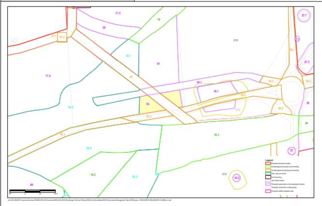
A proposed stockpile area located between the existing A303 and the temporary road to Winterbourne Stoke crossroads. The site is bisected by a utility corridor (Site 49).
