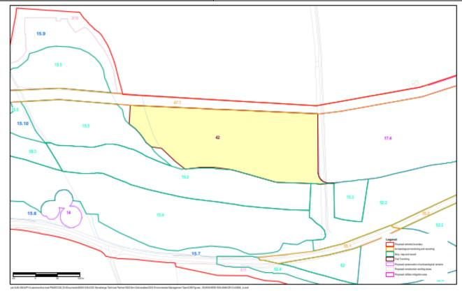
Site 42 is a rectangular area of approx. 5.5ha. west of Longbarrow Roundabout (includes part of the utility corridor (Site 47) that crosses the site). The area lies within the Main Civils Compound site and is required for construction of the Tunnel Production Area (temporary segment production plant, and an associated storage area, batching unit and slurry ponds) and excavated material processing area.
