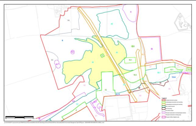
Site 44 is a large irregular area at Parsonage Down, (approx.7.9ha. in size) that contains within it an area for archaeological excavation and recording (AER) (Site 11) and part of the existing Esso Pipeline and its proposed realignment (Sites 46.1 and 46.2) along its eastern flank.
