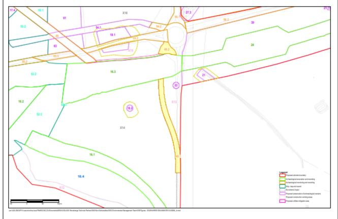
Site 48 comprises the indicative route of the proposed temporary diversion of the A360 via a temporary bridge over the new A303 cutting. The diversion route would also be followed by the proposed temporary and permanent power connection to the Main Civils Compound and Western Portal. The underground cable
